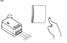
Whilst the indicator on the receiver flashes, press the Kinetic switch ONCE to complete the pairing.
